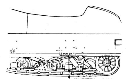
WARNING: Too much tension will result in power loss and excessive stresses on suspension components.
